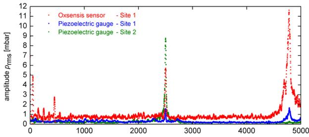
Figure 5: Oxsensis and DLR test results ref [1]
